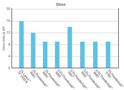
Addition level 2% on total formulation weight for Lanco™ TF 1830 N, PowderAdd™ 9083 and PowderAdd™ 9084 and 0.5% for PowderAdd™ 9085, PowderAdd™ 9567, PowderAdd™ 9082 and PowderAdd™ 9680 and 5% PowderAdd™ 9780.
