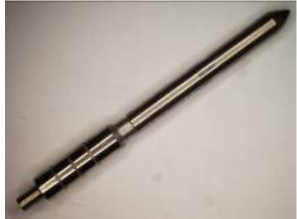
Figure 20 Additized ‘keep clean’ run injector needle
