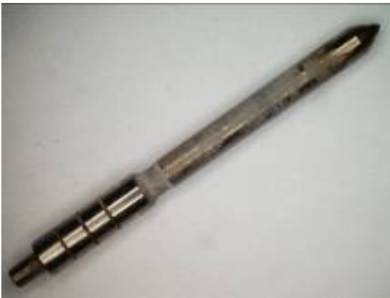
Figure 19 Base fuel fouling run injector needle.
