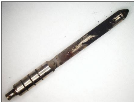
Figure 14 Image of sticking injector from OEM 2 Tier 3 common rail engine.
