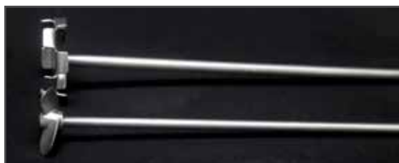
Propeller or dissolver for dispersing Carbopol® polymers.
