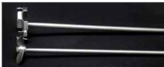
Propeller or dissolver for dispersing Carbopol® polymers.
