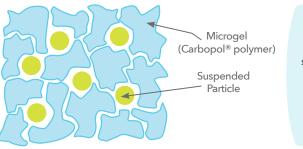
Carbopol® polymers offer superior suspending ability with minimal sedimentation owing to high yield value rather than viscosity.
