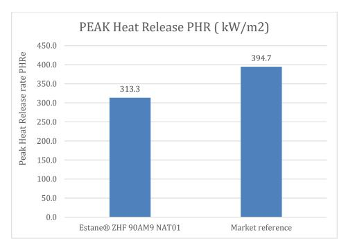
Sample thickness: 3 mm. & Irradiance level: 35 kW/m2
