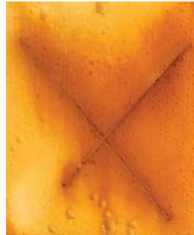
Commercial Benchmark 2 shows corrosion and blistering across the whole panel
