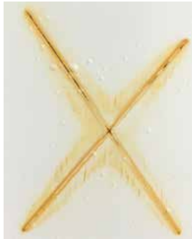
Commercial Benchmark 1 shows more corrosion and blistering around the scribe
