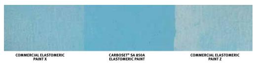
CARBOSET® SA 850A SHOWS EXCELLENT EFFLORESCENCE RESISTANCE COMPARED WITH TWO COMPETITIVE BLUE COATINGS.
