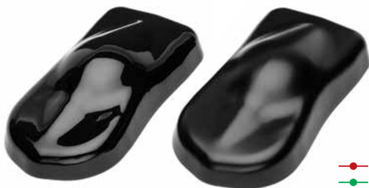
Aptalon™ M8100 gloss formula and Aptalon™ W8030 formula with no matting additives.
