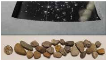
250-300 Stones @ 30-60 MPH via Gravelometer Test (*In accordance with SAE J400)
