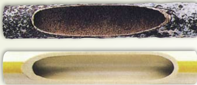
Lubrizol's TempRite CPVC does not corrode like traditional, non-plastic piping systems, as shown in these pipe cutaways.
