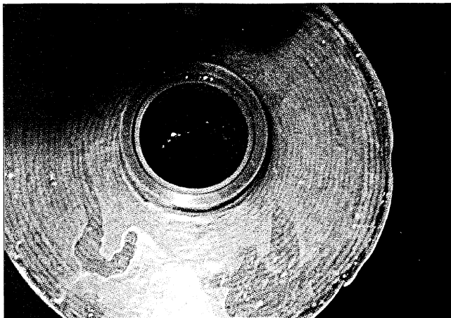
Figure 2. RO membrane fouled with iron and copper sulfides.
